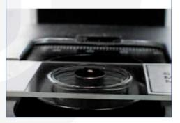
2. Turn the condenser to the highest position and place a drop of immersion oil on the lens
