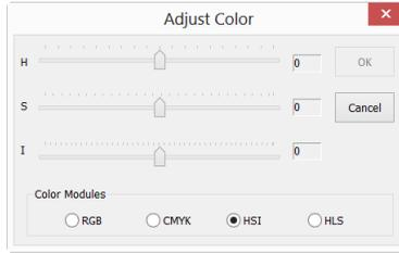
**Hue** is the color reflected from or transmitted through an object. It is measured as a location on the standard color wheel, expressed as a degree between  $0^\circ$  and  $360^\circ$ . In common use, **Hue** is identified by the name of the color such as red, orange, or green.
