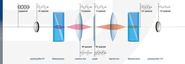
By passing a second Nomarski-modified Wollaston prism, the spatially shifted polarized light is recombined. These recombined light rays pass through a second polarization filter that blocks useless direct transmitted light. The interference of the two rays is sensitive to the optical path difference and by introducing an adjustable offset, the contrast is proportional to the path length so that the heights
