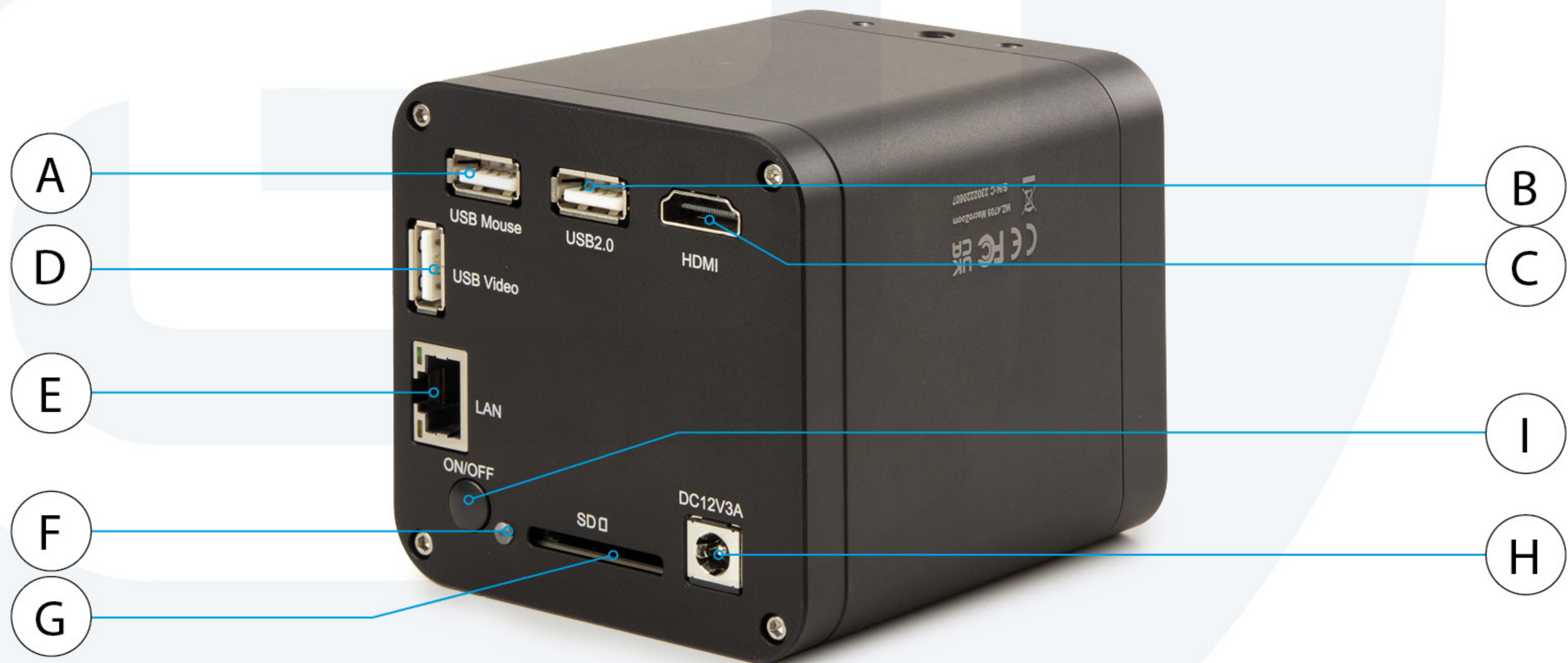
Available ports on the back panel of the camera body
